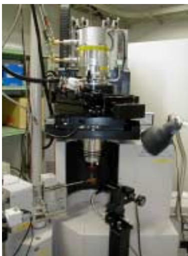
Fig.1 Weissenberg type imaging plate equipped with the helium closed-cycle refrigerator. High-pressure and low-temperature single crystal structure analysis can be performed.
