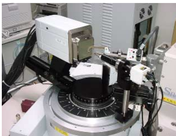
Fig.2 CCD area detector for single-crystal structure analysis with high sensitivity and high accuracy in the temperature range of 90-300K.
